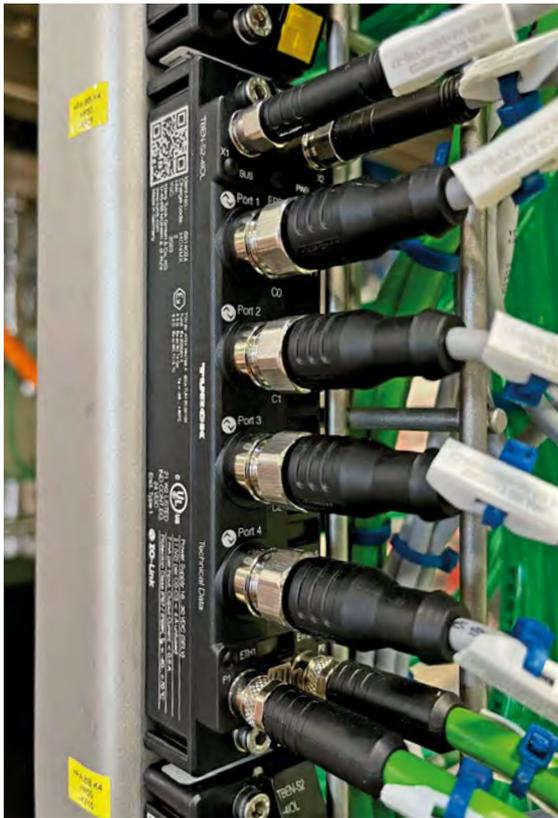
Masterclass: Turck's IO-Link Master TBENS2-4IOL enables the efficient use of IO-Link and digital I/Os in an ultra-compact assembly group at the process node for cooling the machine
