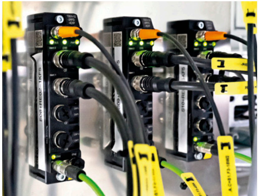
Turck's TBEN RFID interfaces with IP67 protection are screwed onto a metal panel in a cabinet-free installation in the warehouse
