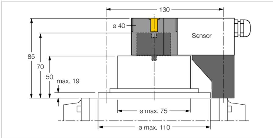
Mounting kit for larger rotary actuators:
