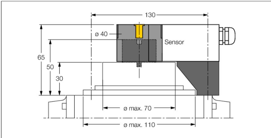
Mounting kit for larger rotary actuators:
