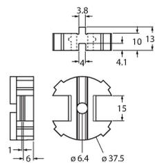
Spacer for dual sensor actuation kit BTS-DSC26-EB20
