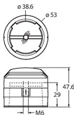
Actuator (puck) for dual sensors; end position damped; hole pattern on flange: 80 x 30 mm and 130 x 30 mm; connection shaft (shaft extension) height: 30 mm/Ø: max. 35 mm; available as an option: Spacer BTS-DSC26-UR10 for 20-mm-high connection shafts (shaft extension)
