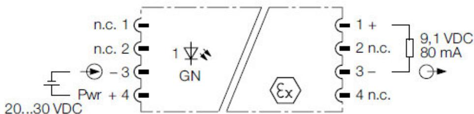
**Figure 6: Block diagram - IMC-DO-11Ex/L/K62**
