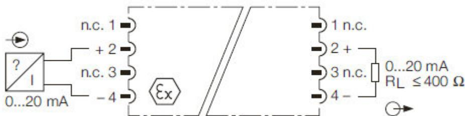
**Figure 1: Block diagram - IMC-AI-\***
