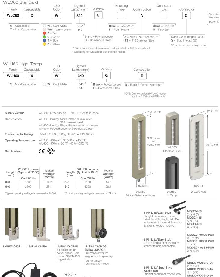
PSD-24-4 Class 2 Power Supply Input: 90-264 V ac 1.5A Output: 24 V dc 3.9A 2 m (6.5') 4-Pin Euro Connector
