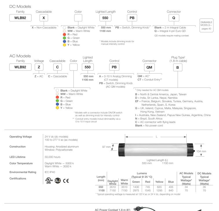
for use with models using QM connector. Cascadable model cables available on page 19.
