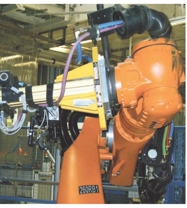
When changing tools on robots, standard Ethernet start-up times of up to 500 ms are unacceptable. BL remote allows tools to be changed more quickly in the subnet before it is connected to Ethernet/IP or Profinet at the robot stand
