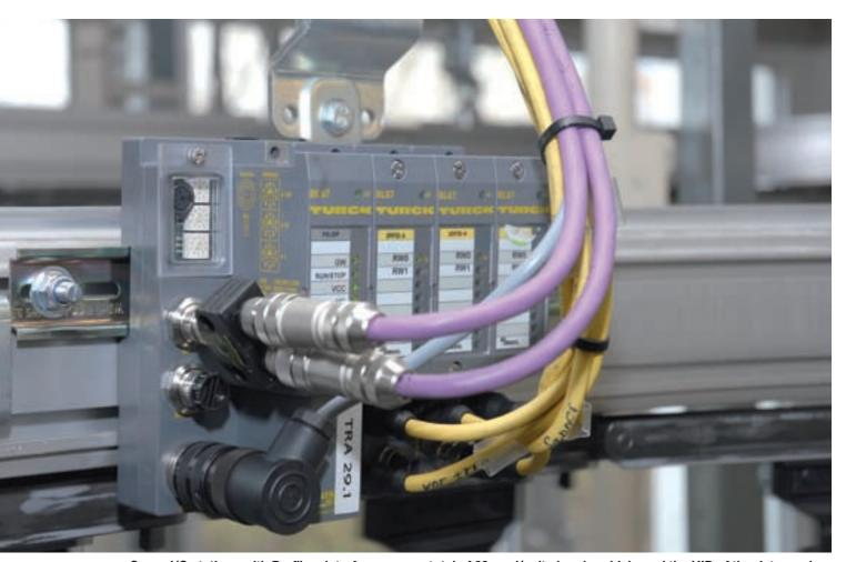
Seven I/O stations with Profibus interface cover a total of 28 read/write heads, which read the UID of the data carriers
