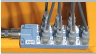
Turck boxes with rapid plug-in systems on Wumag's aerial work platforms are extremely leakproof Page 32
