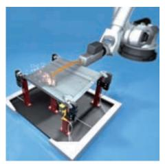
After release by the PLC, the welding robots score the nuts and bushings on the sheet metal
