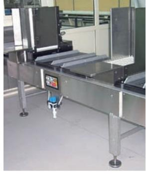
At the changing station the machine operator can introduce molds for a new batch and eject the old ones. Every movement is directly recorded in the central database
